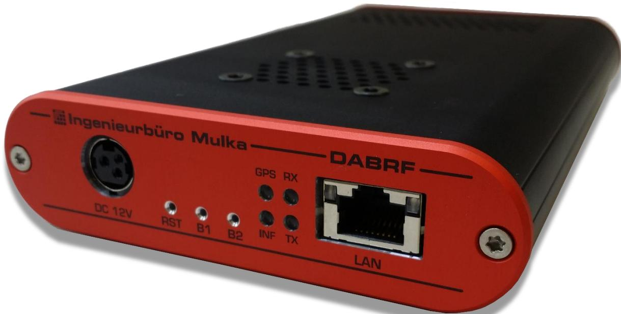
*Figure 6 – DABRF-HWU receiver and modulator*
