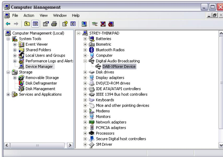
Figure 41 – Device manager showing the DAB-XPlorer (DABXP-HWU) as a new device
